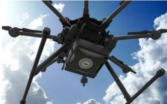
operations group in the remote area to the field. The solution is a tethered drone, a private LTE picocell, offering an extensive coverage footprint (approx. 20 miles) in the remote areas to in-field users for voice, data, and sharing the backhaul with mobile surveillance video system, radar, and critical apps running on data devices such as tablets and smartphones. AGILE Virtual SIM device provides the ability to manage a library of multiple SIM cards from large cellular LTE and
