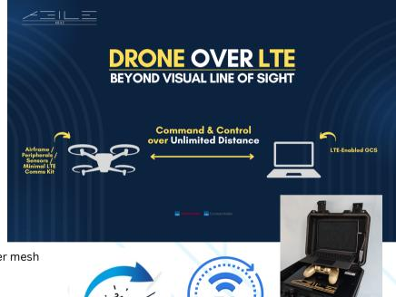
The CORE of the system is an open-source autopilot platform that integrates with LTE 5G for communication. This setup ensures a reliable and continuous connection between the vehicle and the control station, leveraging the widespread LTE 5G infrastructure for global coverage. The open-source nature of the autopilot software encourages continuous development and customization, making the system versatile across various applications.
