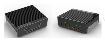
Our devices automatically search for the best throughput connection available. If all LTE connections are lost, Mobile CORE X1 can connect to any available satellite modem. If the device finds an available cellular connection it will reconnect to that service, hands-free. The customer does not have to monitor AGILE Routing.
